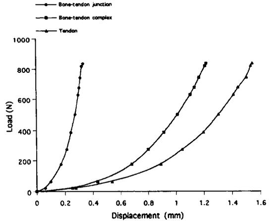
**Fig. 2** Plot of load against displacement for tendon, bone-tendon complex and bone-tendon junction. Test was performed at 45° and 12 mm min<sup>-1</sup> of displacement rate
