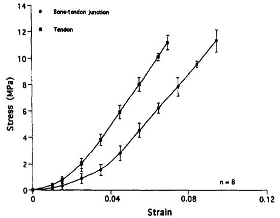
**Fig. 6** Engineering stress-strain curves of tendon and bone-tendon junction at 90° of loading. Statistical analysis (Two-way ANOVA test) revealed that there are significant differences in strains of tendon and bone-tendon junction ( $P < 0.05$ )
